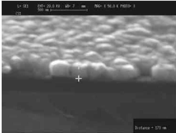
Figure 19: SEM micrograph of a copper film electrodeposited from bath 1 at 0.5 \text{ mA/cm}^2 .
