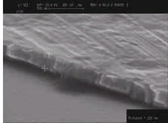
Figure 7: SEM micrograph of a [Cu(7.5nm)/CoNi(Cu)(3nm)] 40 ML grown onto Si/SiO 2 /Cr(70nm)/Au ECD flash (substrate E).
