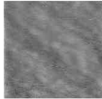
Figure 5: AFM micrograph of Si/SiO 2 /Cr(70nm) substrate with Au ECD flash (0.5μm x 0.5μm).
