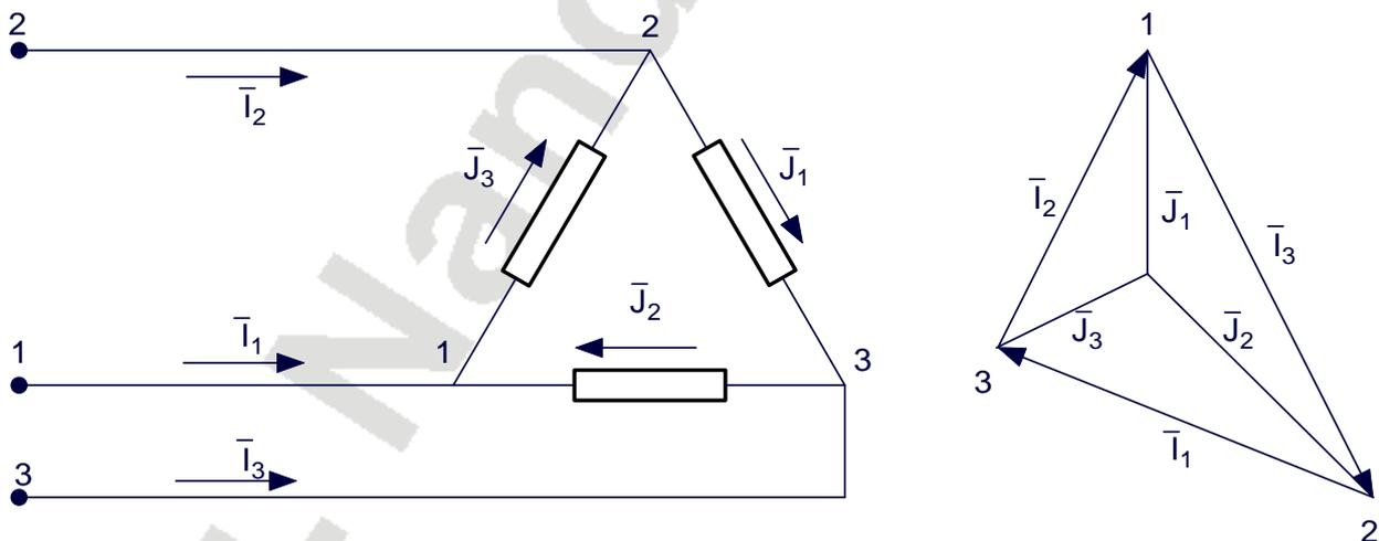
$$\begin{aligned}\bar{I}_1 &= \bar{J}_3 - \bar{J}_2 \\ \bar{I}_2 &= \bar{J}_1 - \bar{J}_3 \\ \bar{I}_3 &= \bar{J}_2 - \bar{J}_1\end{aligned}$$
