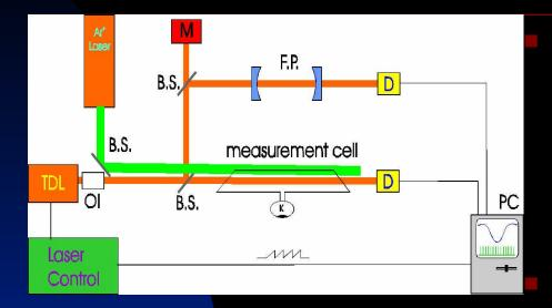
The effect has been monitored by diode laser absorption spectroscopy on the potassium D<sub>1</sub> line at 770 nm;
