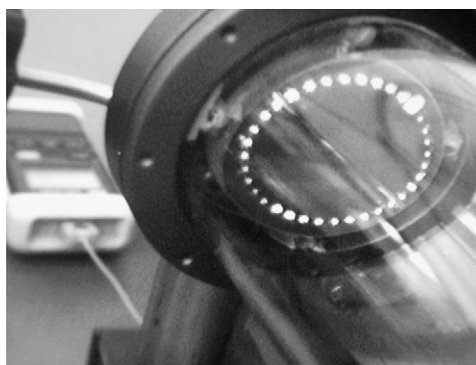
Fig. 2. A particular of the laser diode beam reflections on one of the two mirrors of the multipass Herriott type cell.
