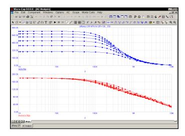
Figure 9-5 AC analysis linear stepping
