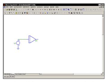
Figure 11-4 The INT macro used in a circuit
