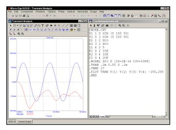
Figure 8-11 Probing SPICE circuits
