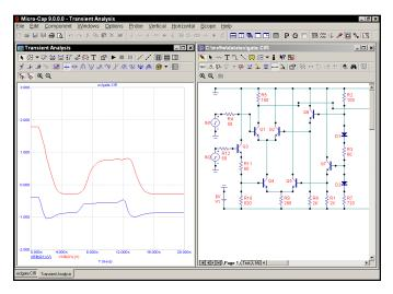
Figure 8-2 Probing lead-to-lead voltages
