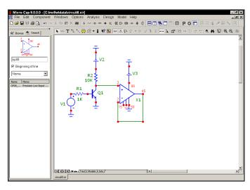
Figure 3-8 The circuit after wiring the OP08
