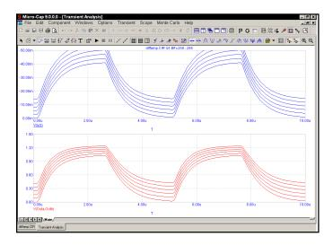
Figure 9-3 Stepping BF in a single transistor
