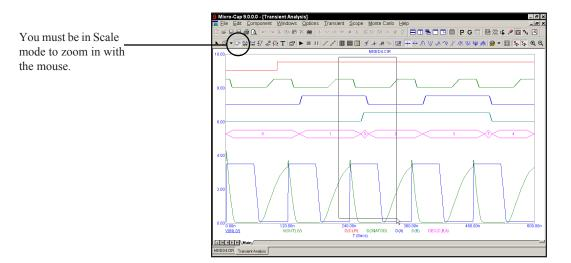
Figure 2-4 Using the mouse to magnify a waveform
