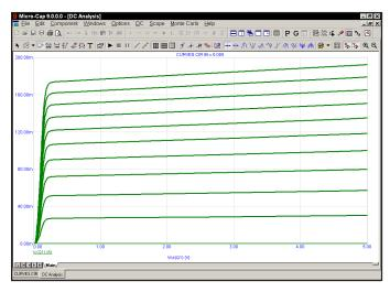
Figure 2-16 The IV curves of a bipolar transistor
