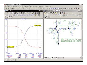
Figure 8-9 DC transfer function plot
