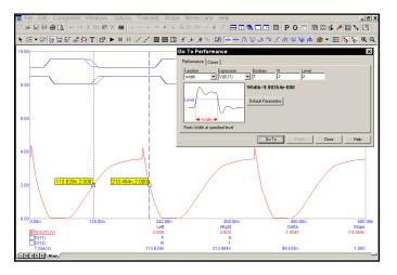
Figure 7-21 Measuring the pulse width
