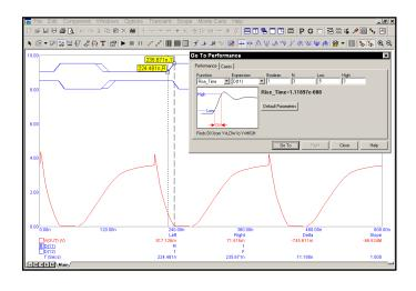
Figure 7-24 Measuring digital rise times
