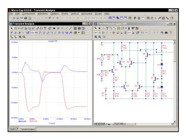
Figure 8-3 Probing lead currents
