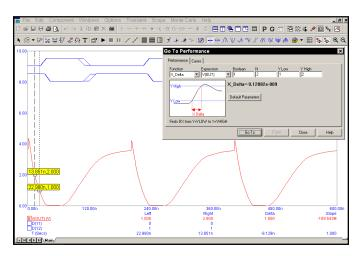
Figure 7-22 The X Delta function
