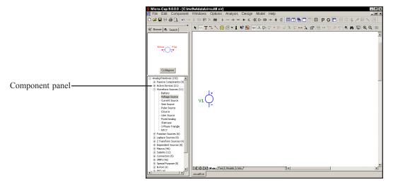
Figure 3-1 Selecting a part from the Component panel
