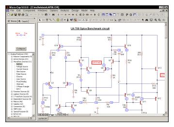
Figure 3-17 The UA709 circuit
