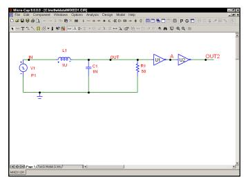
Figure 4-10 The MIXED1 circuit
