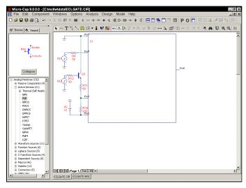
Figure 11-7 The ECLGATE circuit using a macro
