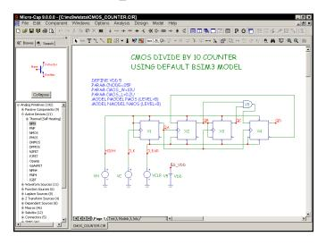
Figure 8-12 The CMOS Counter
