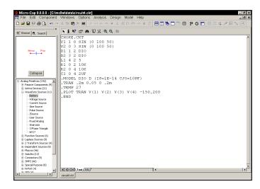
Figure 3-21 The sample SPICE circuit
