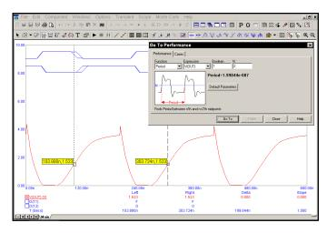
Figure 7-20 Measuring the pulse period
