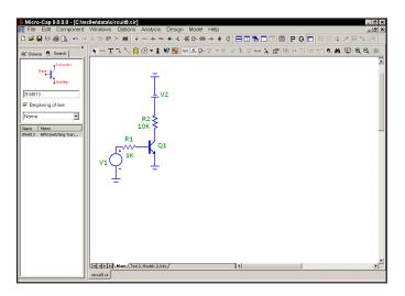
Figure 3-7 The circuit after adding the bipolar stage
