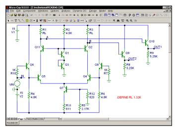
Figure 2-10 The RCA3040 circuit
