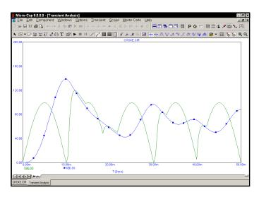
Figure 7-2 Transient analysis of the CHOKE circuit
