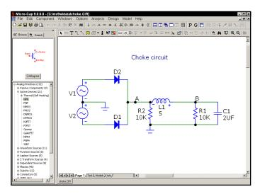
Figure 7-1 The CHOKE circuit
