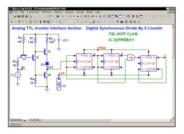
Figure 2-1 The MIXED4 sample circuit
