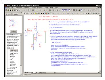
Figure 12-4 Using the subckt component
