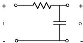
$$H(j\omega) = \frac{1}{1 + j\omega RC}, \quad \omega_t = \frac{1}{RC} \text{ rad/s}$$
