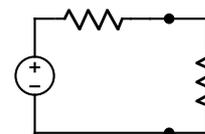
$$P_R = \frac{36R}{(R + 5)^2} \text{ W}, \quad R_{ad} = 5 \Omega$$
