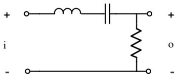
$$H(j\omega) = \frac{j\omega RC}{1 + j\omega RC - \omega^2 LC}$$
