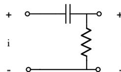
$$H(j\omega) = \frac{j\omega RC}{1 + j\omega RC}, \quad \omega_t = \frac{1}{RC} \text{ rad/s}$$
