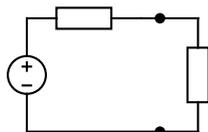
$$Z_{\text{ad}} = Z_s^* \Omega, \quad P_{\text{ad}} = \frac{|\dot{V}_s|^2}{8R_s} \text{ W}$$
