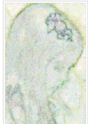
This image shows the (accentuated) difference between an image saved as JPEG and the original. Note especially the changes occurring near sharp edges.
