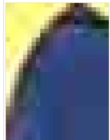
The compressed 8x8-squares are visible in the scaled up picture, together with other visual artifacts of the lossy compression
