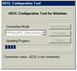
Back on the front screen click on Apply to send the new settings across to the router. The router will automatically reset after the new settings have been uploaded.
