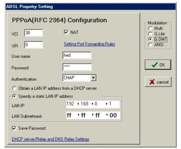
For normal UK operation select PPPoA (RFC 2364) as the Connection Mode and then on Properties to set the router settings:
