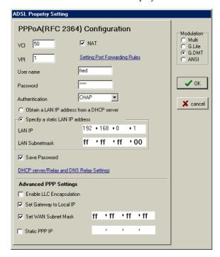
For operation on a KC ADSL line tick the box 'Enable LLC Encapsulation'.
