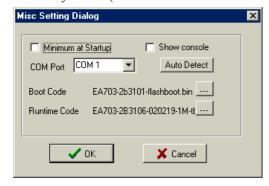
Now click with right-mouse-button on the ADSL Configuration Tool startup window and then select Misc Setting from the drop down menu shown:
