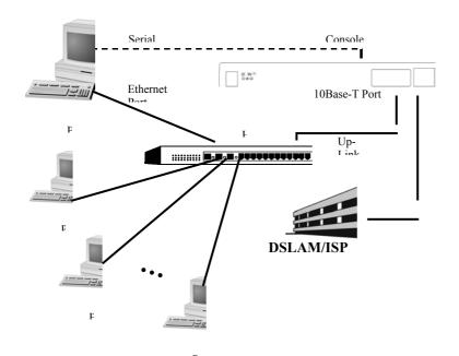
The LAN port on the SAR router is the type designed to be connected to an 'uplink' (or crossover) port on a hub. This means you can also connect the router LAN port direct to the port on a PC LAN card using a standard cat5 LAN cable. If you wish to connect the router to a 'normal' port on a hub then you will need to use a crossover cable or adapter.
