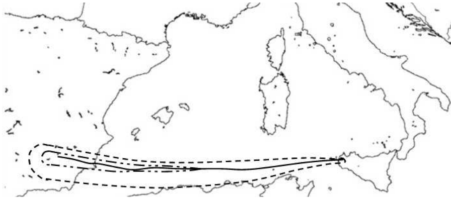
Fig. 8. Example of preflight (dashed line) and mid-flight (dashed-dotted) simulations for a balloon flight (solid line)
