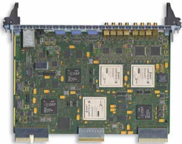
Figure 2 – Xilinx Virtex-5 FPGAs reside on the LSU’s software-defined radio card, along with TI DSPs.
