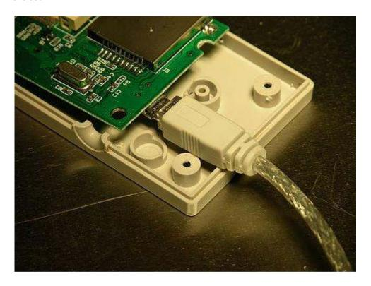
He placed the card reader in the controller after gluing some buttons in place. He however faced problems while attaching the cord for the card reader. Soldering a new USB cord in proved quite impossible too. Hence, he cut away some parts of the plastic though it meant taking some risk.
