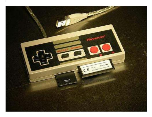
The Dremel tool, hobby knife set and the glue were used for making the work easier. The card reader is just about the same size as that of the Nintendo controller. This makes things easier and soldering and opening things up can be avoided.
